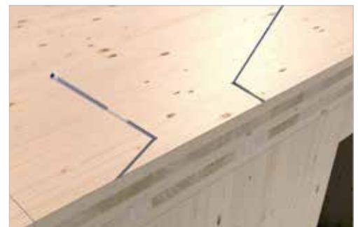
SWD inclined installation of CLT floor panels.
