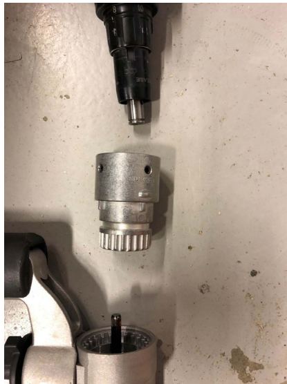
DWA3G2 adaptor installed and small screws tighten with the allen key.
