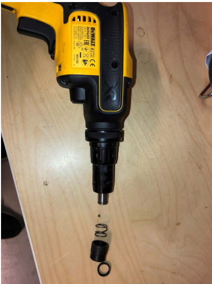
Remove the metal ring in front of the nosepiece on the power tool.
