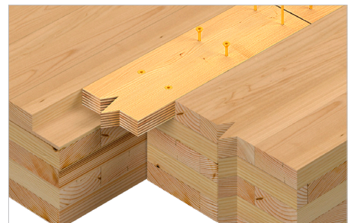
ESCRC screw installed into a CLT spline.
