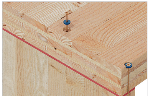
ESCR screw installed into a CLT floor-to-wall connection.
